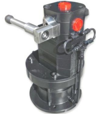
The torque is developed by one power piston and is transferred to the output shaft with a second also contact free rotating piston by a synchronising gear train.
